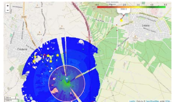
Figure 2: Overlapping of theoretical LoRaWAN coverage vs actual on-site measurements at Intracom Telecom campus
